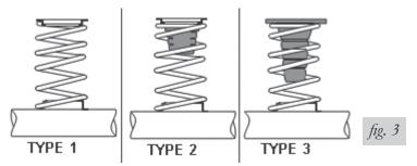
**Type 1:** If there is no jounce bumper at top spring seat (see fig. 3), and there is a large hole, insert the protector and cylinder so stem is up. See Figure 5.
