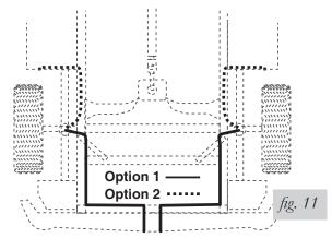
2. Determine and cut adequate length of air line to reach from valve location to left side air cylinder.
