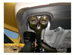
3) Place a supplied clamp onto the left muffler outlet. Place the left tailpipe **#26564H** into position and starting from the rear, connect the hangers on the tailpipe to the rubber mounts on the vehicle. Slide the tailpipe fully into the muffler outlet. Adjust the tailpipe so that the stainless tip is level and centered in the bumper cut-out. Tighten clamp enough to hold, but still allow for adjustment. Repeat this step for right tailpipe **#26563H**.
