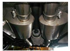
2) Place a supplied 3" clamp onto the inlet neck of both mufflers. Slide the mufflers onto the back of the Scavenger X-pipe assembly and support with stands. Level the mufflers and tighten the clamps enough to hold, but still allow for adjustment.
