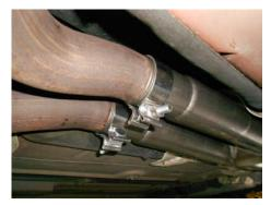
1) Begin the installation by placing a supplied 2-3/4" clamp onto each of the inlets of the X-pipe assembly **#26576H.** Then, place the X-pipe onto the back of the stock head pipes (the embossed Hurst H will be facing the ground). Level and center the assembly in the drive line tunnel and support with a stand. Tighten the two clamps enough to hold, but still allow for adjustment.
