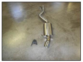
1) Place the new Hurst muffler units next to the factory units and swap the front and rear hanger mounts from the stock mufflers to the Hurst assemblies. Also, place a provided 2.25" clamp onto the inlet of each assembly. Tighten the clamp just enough to hold in place.
