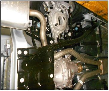
2) On convertible model vehicles, the body braces shown in the photos above will need to be removed in order remove the factory system and install the Hurst system. Starting at the front of the right side (passenger) brace, loosen the front bolt and then work your way to the rear of the vehicle removing the next eight bolts. Once the bolts have been removed, lower the brace from the vehicle. Repeat this step on the left side of the vehicle with the six bolts on that side.
