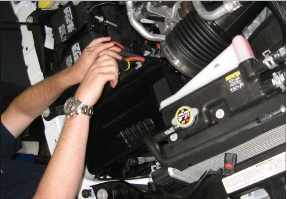
Figure 6-Removing bolt that secures air filter housing to vehicle
