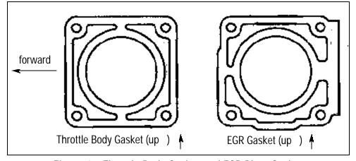
Figure 1 – Throttle Body Gasket and EGR Plate Gasket
