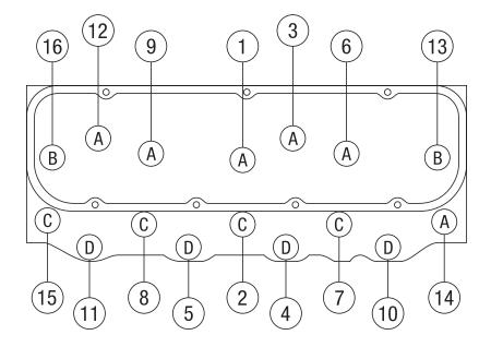
Figure 1 - Big Block Chevrolet Cylinder Head Bolt Torque Sequence Torque Bolts to 70 ft./lbs. (Torque Bolts in 3 to 4 steps, gradually approaching final torque spec)
