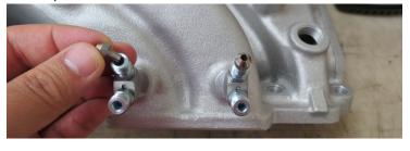
2. Install the passenger side Nitrous Assembly (Blue Assembly) onto the E2 nozzles. Nozzles are marked "N" for nitrous and "F" for fuel. Hand tighten all fittings, then use a 7/16" wrench to snug down the fittings.
