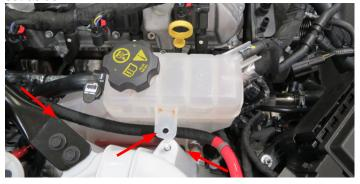
53. Using a panel puller, remove the engine harness from the support bracket located on the passenger side valve cover.
