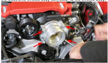
102. Using a 10mm socket, remove the EVAP solenoid from the stock manifold. Inspect the o-ring gasket and replace if needed.
