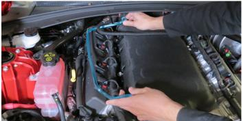
27. Disconnect the brake booster line assembly from the iunction on the driver side strut tower.
