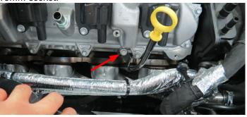
58. Remove five (5) bolts securing the passenger side exhaust manifold to the cylinder head. Carefully remove the exhaust manifold along with the dipstick. Discard the exhaust manifold gasket.
