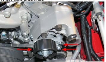
78. Position the ground strap behind the engine harness bracket and secure the engine harness to the cylinder head. Reconnect the engine harness.
