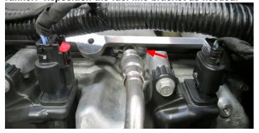
92. Connect the supplied 1/4" hose to the actuator barb on the driver side runner. Route the hose over towards the passenger side runner and towards the front of the vehicle. *TIP: Make sure to tuck the hose along the bottom of the passenger side runner as to clear the supercharger manifold.*
