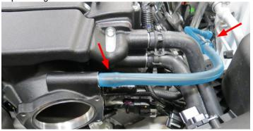
129. Connect the supplied EVAP hose to the hardline on the firewall. Route the hose over towards the driver side strut tower and connect it to the EVAP solenoid.
