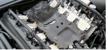
41. Using a Torx T30, loosen the passenger side coil cover and remove the 2nd and 4th valve cover bolts with a 10mm socket. Secure the side cover brackets to the valve cover with the stock valve cover bolts.
