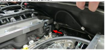
94. The MAP connector will route behind the driver side runner and connect to the factory MAP connector. NOTE: Some factory MAP connectors will have a inner left tab which will have to be trimmed. The two MAF connectors on the TMAP harness will connect to the MAF sensor and the factory MAF connect later.
