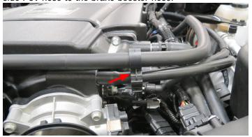
132. Connect the MAF connector from the TMAP harness to the MAF sensor and the factory MAF connector.
