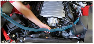
22. Disconnect the electronic throttle body connector from the throttle body.
