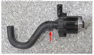
73. Install the supplied water pump isolator onto the water pump noting the orientation.
