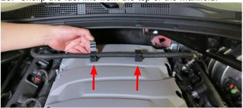
24. Using a deep 10mm socket, remove four (4) bolts securing the manifold cover.
