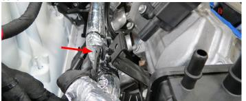
54. Using a 10mm socket, remove the engine harness support bracket.
