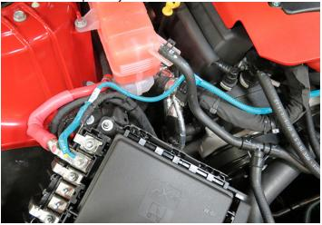
136. Remove the factory GROUND terminal nut attached to the chassis. Attached the GROUND connector on the water pump harness to the chassis ground and secure with the factory terminal nut. Remove the nuts securing the fuse box to the chassis. Gently remove the fuse box from the mounting studs and secure the relay to the mounting stud. Reinstall fuse box nuts.
