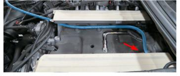
93. Connect the TMAP harness to the TMAP sensor located on the inside of the passenger side runner. Route the harness towards the front of the vehicle, along the valley side of the driver side runner.
