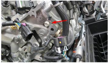
80. Install the supplied tensioner onto the FEAD bracket using three (3) M8 x 40mm bolts from hardware bag #1. Torque bolts to 22 ft-lbs.
