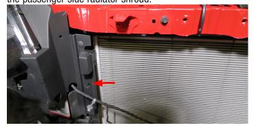
112. Using a panel puller, remove both inner push pins securing the right and left air ducts.
