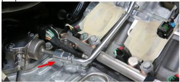
35. Loosely secure the fuel line extension to the valve cover using the factory bolt. Apply Blue thread locker to the threads of the fuel line extension lock nut. Using a 11/16" wrench, secure the fuel line extension to the fuel pump using the lock nut. Tighten the lock nut, **DO NOT OVER TIGHTEN**. Securely fasten the fuel line extension support bracket to the valve cover using the factory bolt.
