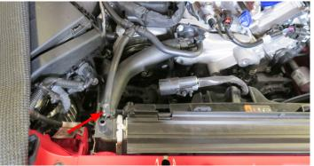
47. Using a hose clamp removal tool, detach the lower passenger side radiator hose. *NOTE: The clamp may not come off because of adhesive. Simply compress the clamp and pull the hose simultaneously.*
