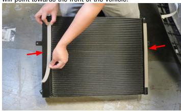
114. Position the LTR in front of the radiator assembly with the inlet barbs positioned on the driver side of the vehicle. Using the supplied push pins from hardware Bag# 2, secure the LTR to the radiator shrouds.
