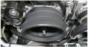
64. Using a 24mm socket and a torque wrench, install the used factory balancer bolt and torque it to 240 ft-lbs. Then remove the factory balancer bolt and discard.
