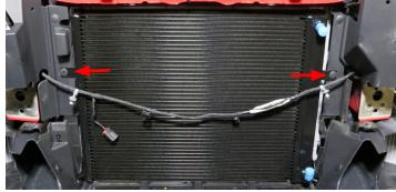
115. Secure the lower portion of the LTR to the air ducts using two (2) M6 x 16mm bolts and two (2) M6 locknuts from hardware Bag #2.
