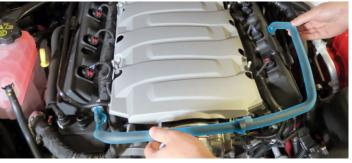
20. Using a 10mm socket, remove the nut securing the noise generator to the firewall.
