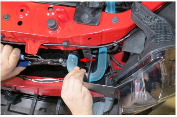
120. Using a 3/4" hose clamp from Bag #2, secure the hose to the lower water crossover barb.
