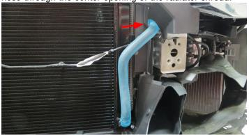
118. Using a 3/4" hose clamp from Bag #2, secure the LTR to Water Pump hose to the outlet barb of the water pump.
