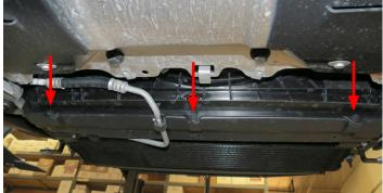
40. Re-install the bolts removed from the previous step with the side cover brackets as shown.
