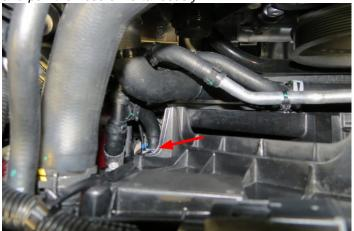
48. Remove the retaining clip securing the transmission cooler line to the radiator and remove the transmission cooler line. NOTE: Be extremely cautious not to drop or lose this clip. Keep the clip in a safe place to be re-installed later.
