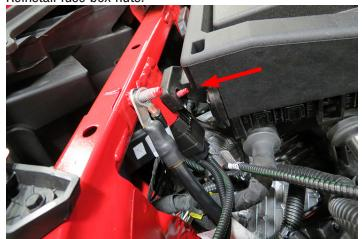
137. Route the EVAP connects over towards the EVAP solenoid. Connect the factory EVAP connector to the EVAP connector on the water pump harness. Connect the EVAP connector on the water pump harness to the EVAP solenoid. TIP: Note connector orientation.
