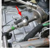
34. Install the supplied fuel line extension onto the fuel pump barb.
