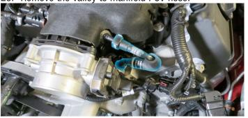
26. Remove the EVAP line from the hardline located on the firewall and from the EVAP solenoid.
