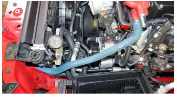
121. Using two (2) 3/4" hose clamps from hardware Bag #2, secure the Surge Tank to Manifold hose to the surge tank and upper water cross over barb.
