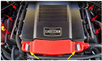
146. Install the side covers onto the side cover brackets.
