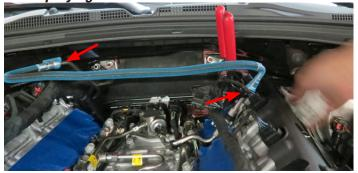
33. Using a 10mm socket, remove the bolt securing the fuel line extension to the valve cover. Remove the retaining clip on the fuel line extension. Then remove the fuel line extension from the fuel pump using a 3/8" fuel line tool.
