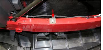
126. Reattach the harness to the crash beam and reinstall the front fascia reversing the disassembly procedure.
