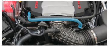
18. Using a hose clamp tool, remove the noise generator hose from the inlet elbow. Loosen the warm clamps securing the inlet elbow and remove the elbow.
