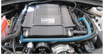
131. Using the factory hose retainer clip, secure the drive side PCV hose to the brake booster hose.
