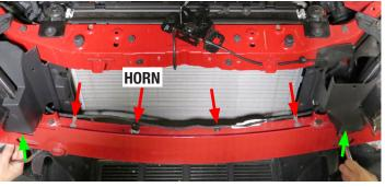
107. Using a 10mm wrench and a 13mm socket, remove ten (10) bolts, five (5) per side, securing the crash beam to the chassis.
