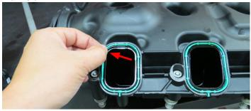
88. Clean and inspect the O-ring gaskets. Replace torn or damage O-rings as needed. Using a razor blade remove the tips off all eight (8) factory O-ring gaskets.
