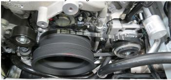
71. Install the factory accessory drive belt using the routing diagram below.
