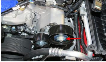
79. Install the supplied tensioner bracket to the provisions on the cylinder head and engine block using two (2) M10 x 100mm bolts and two (2) M8 x 55mm bolts supplied in hardware Bag #1. Torque M10 bolts to 32 ft-lbs and M8 bolts 22 ft-lbs.
