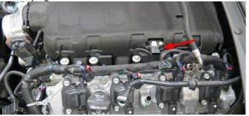
29. Using a 10mm socket, remove ten (10) bolts securing the intake manifold to the cylinder heads. Carefully remove the intake manifold assembly.
