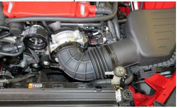
134. Using a razor blade or equivalent, remove the 90° fitting from the factory air inlet PCV hose. Connect the fitting to the supplied air inlet PCV and attach the straight quick connect to the air inlet and the 90° quick connect to the center PCV junction.
