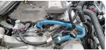
87. Remove the factory 0-ring gaskets from the intake manifold.
