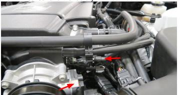
133. Using the supplied worm clamps, secure the inlet elbow to the throttle body and the air intake box.
