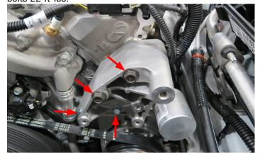
82. Install the smooth idler pulley to the upper water pump provision and the smaller grooved idler to the lower water pump provision. Torque both bolts to 22 ft-lbs.
