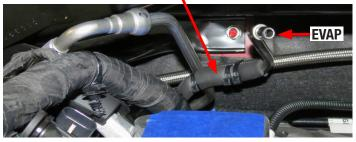
84. Connect the supplied fuel feed line to the hardline on the firewall and route it over towards the fuel adapter line. Secure the fuel line to the brake line with wire ties.
