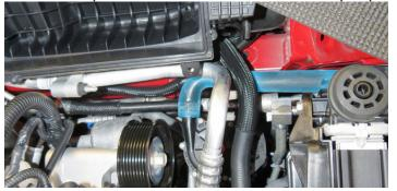
119. Route the LTR to Manifold hose through the hole in the radiator shroud and back towards the manifold. Using a 3/4" hose clamp from Bag #2, secure the hose to the upper barb of the LTR.
