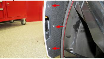
12. Use a 7mm socket to remove six (6) screws securing the corner of the fascia to the fender; three (3) per side.
