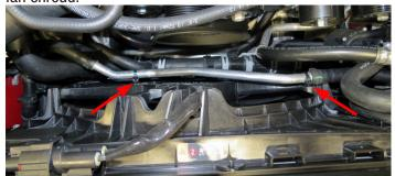
50. Remove four (4) bolts securing the electric fan to the radiator using a 10mm socket. Carefully remove the electric fan assembly.
