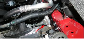
49. Using a panel puller, remove the coolant lines from the fan shroud.
