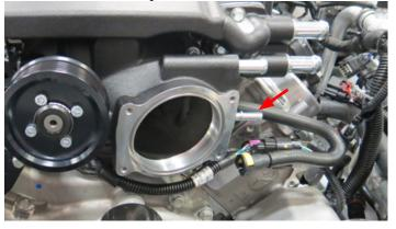
99. Using a breaker bar, rotate the tensioner counterclockwise and install the supercharger belt using the routing diagram below.
