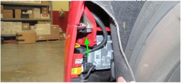
13. Pull back the wheel liner and remove eight (8) additional screws securing the fascia to the fender; four (4) per side. *NOTE: Fourth bolt not shown, location is above top bolt.*
