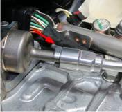
36. Using a razor blade or equivalent, cut out the fuel line relief on the foam valley insulator.
