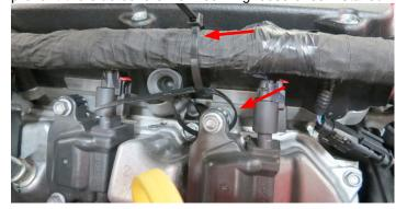
39. Using a Torx T30, remove the driver side coil cover. Using a 10mm socket, remove the 2nd and 3rd bolt from the driver side valve cover.
