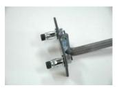
6) Insert the bolt threads through the back of the hanger and install the washers and nuts. Place the assembly into the pair of the holes in the floor as shown in Step 4. Tighten the nuts securely. As you tighten, the jack-nuts will collapse and secure the assembly in place.
