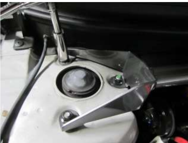
a. Install the AEM Strut Tower Bar, re-install the strut tower nuts, and torque to 43.4 ft-lb.
