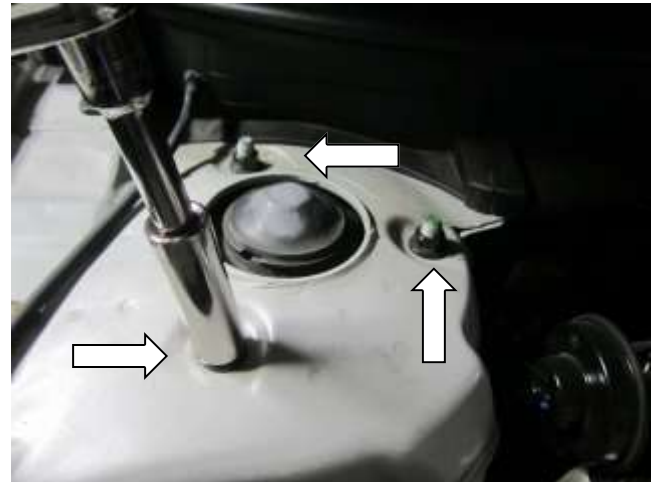
a. Remove the 3 Strut Tower nuts from each side needed to install the AEM Strut Tower bar.
