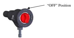
7. When a fuel sample is needed, rotate the red locking knob to the "ON" or unlocked position and press the knob until the desired sample is acquired. After the desired sample has been taken return the red locking knob to the "OFF" or locked position.
