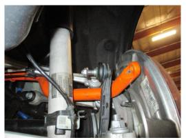
3. Apply a generous amount of supplied grease on the bushing and install on the bar by separating the slit in the bushing. Install the CNC machined aluminum bushing bracket using the OEM E12 Torx bolts. Torque bolts to 25 lb-ft
