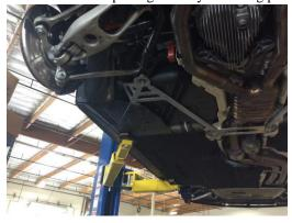
5. Using a T60 torx socket, a T40 torx socket, and a 16mm socket, remove the bolts that hold the rear chassis reinforcement to the body.
