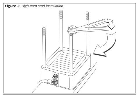
supplied thread locking compound to the M8 threaded end of the studs. Hand tighten the studs to the intake manifold.
