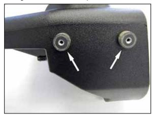
6. Install the two provided rubber mounted studs onto the AEM<sup>®</sup> air filter housing using the provided hardware.
