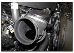
3. Loosen the hose clamp that secures the intake tube to the turbo inlet and then remove the intake hose from the vehicle.
