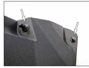
4. Install the two provided mounting studs onto the bottom of the AEM<sup>®</sup> air filter housing using the provided hardware.
