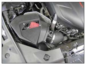
11. Install the provided coupler onto the turbo inlet. Install the AEM<sup>®</sup> filter housing assembly into the vehicle so the mounting studs engage the factory mounting grommets. Connect the intake coupler to
