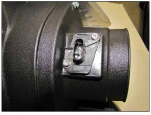
10. Remove the intel air temperature sensor from the factory housing and install it into the AEM<sup>®</sup> housing using the provided hardware.
