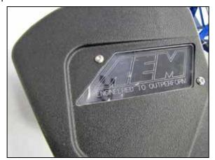
5. Install the AEM<sup>®</sup> window into the AEM<sup>®</sup> air filter housing and secure with the provided hardware.
