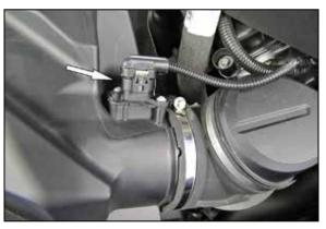
2. Disconnect the inlet air temperature sensor electrical connection and loosen the hose clamp that secures the factory intake tube to the air filter housing. Pull up the air filter housing to release it from the mounting grommets and remove it from the vehicle.
