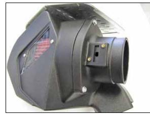
9. Install the temperature sensor housing onto the air filter housing and secure with the provided hardware.
