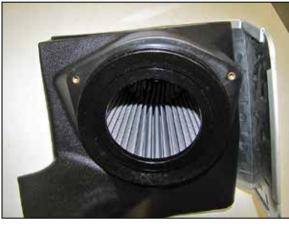
8. Install AEM<sup>®</sup> air filter into the filter housing as shown.
